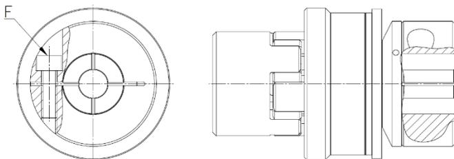
In general, the hubs of the KBK coupling can be installed both separately and in mounted condition. Slide the hubs onto the stub shaft. In the correct axial position, tighten the clamping screw (F) according to the tightening torque stated in the table, by using a torque wrench.
