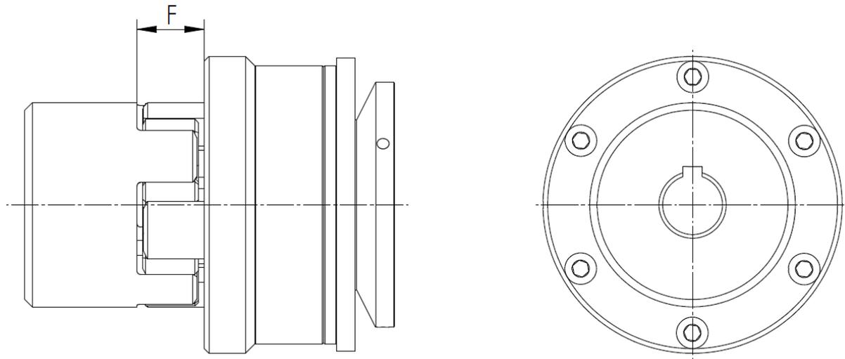
The clearance (F) should be adhered to, to increase the skew compensation of the coupling as well as the durability of the spider. This applies for all safety couplings with elastomer spider elements.
