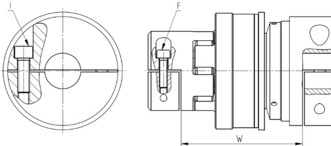
Align the shafts with each other, paying attention to the shaft distance (W). Loosen the split hubs from the coupling and place the coupling on the shafts. Then tighten the split hubs again and tighten the screws (F/I) to the torque stated in the table by using a torque wrench.
