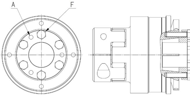
In general, the hubs of the KBK couplings can be installed both separately and in mounted condition. Slide the hub onto the stub shaft. In the correct axial position, tighten the clamping screws (F) evenly and crosswise according to the torque stated in the table, by using a torque wrench.
