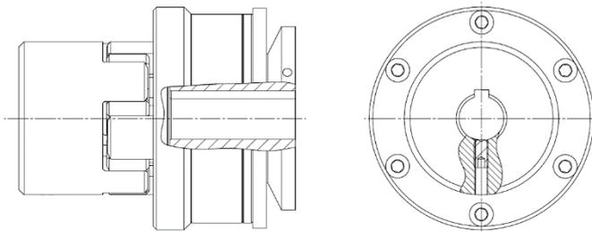
In general, the hubs of the KBK coupling can be installed both separately and in mounted condition. Slide the hubs onto the stub shaft. In the correct axial position, the hub must be fixed against the stop collar or by means of a locking ring. Put the elastomer spider element into the correct axial position and tighten the setscrew.
