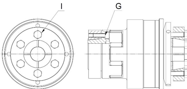
In general, the hubs of the KBK couplings can be installed both separately and in mounted condition. Slide the hub onto the stub shaft. In the correct axial position, tighten the clamping screws (F) evenly and crosswise according to the torque stated in the table, by using a torque wrench.
